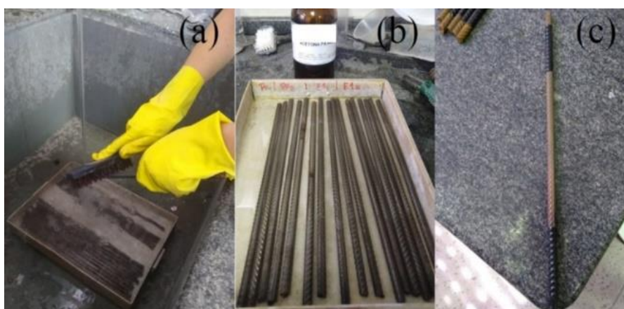
Figure 1 - Washing and brushing of steel bars (a), bars immersed in acetone for quick drying (b), and corrosion area delimitation with electroplater's tape (c).
